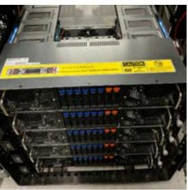
40 GPUs in 5 FIONA8s for ML in 15" of rack space 2.4 Million GPU hours per day
